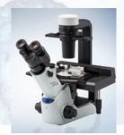
Inverted microscope: is a microscope with light source useful for observing living cells in culture flask
